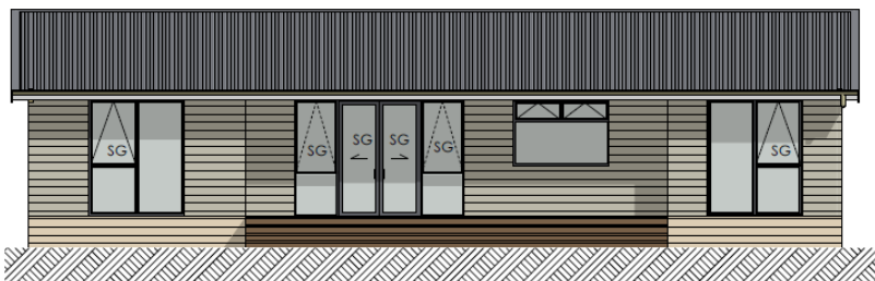
ELEVATION A SG-Indicates Safety Glass
